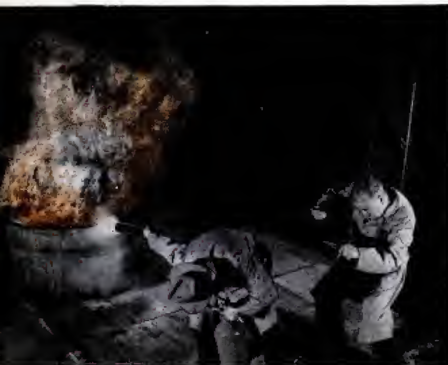
Engineers use a one-quart vaporizing-liquid extinguisher to put out blaze in cotton waste soaked with gasoline. Below, testing a carbon-dioxide extinguisher on a fire made by igniting two gallons of gasoline in a four-foot iron container
